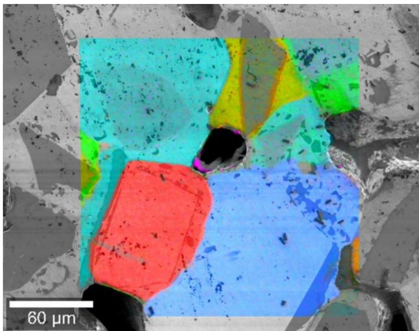
Figure 1: Correlative Raman-SEM (RISE) image of recrystallized silicon carbide (RSiC) ceramics. The SEM image shows the structure, while the Raman image reveals the distribution of various SiC polymorphs.
