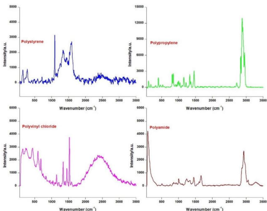
Figure 1: Raman spectra of identified microplastics in the dust
