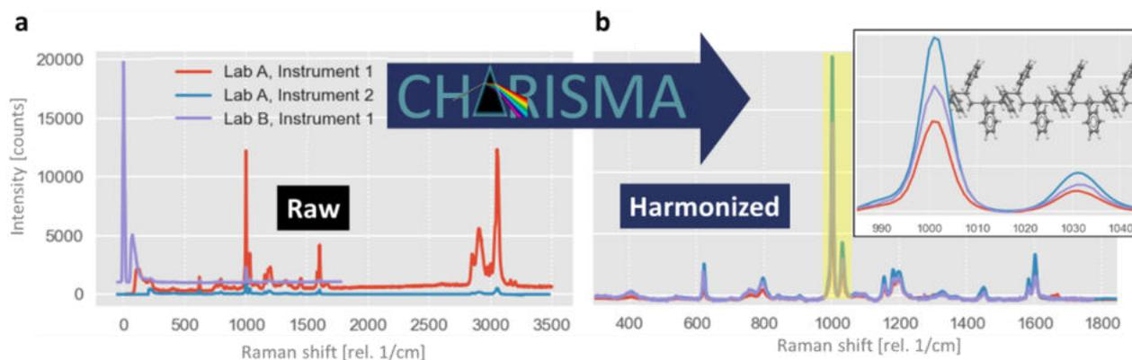
CHARISMA will implement harmonization of raw Raman data from various sources and formats (a) through pre-processing and calibration. Harmonized data (b) can be quantitatively compared, grouped, and used for statistical model development. The example shows spectra of polystyrene, a common polymer (inset in (b)).
