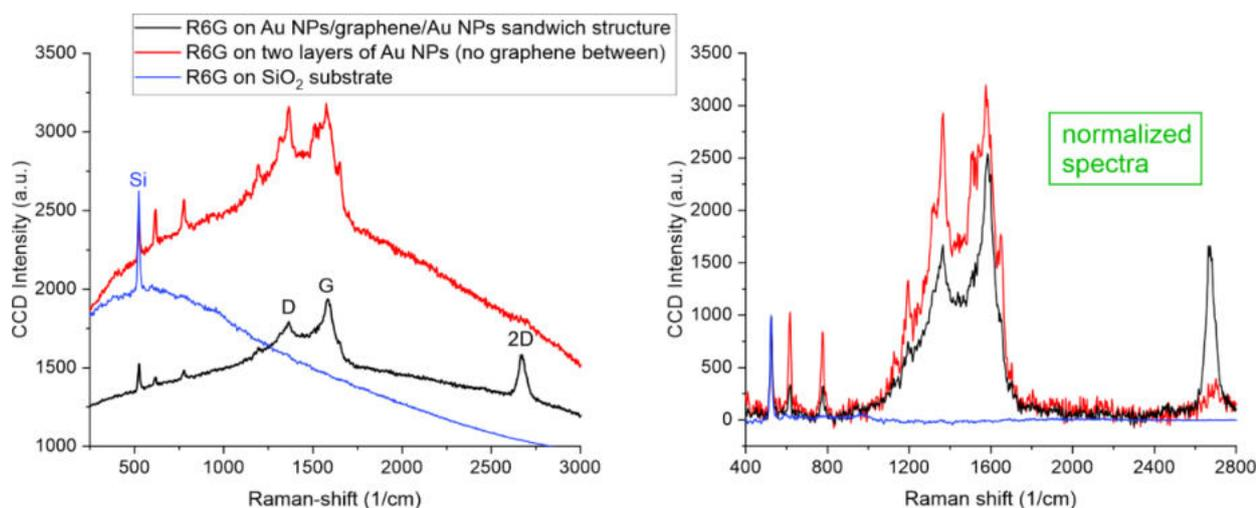
Left: Average Raman spectra of rhodamine (R6G) on the Au NPs/graphene/Au NPs sandwich structure (black), on Au NPs without graphene between (red), and on SiO<sub>2</sub> substrate (blue). Right: the same spectra as left, background-subtracted and normalized to the Si (520 cm<sup>-1</sup>) peak.
