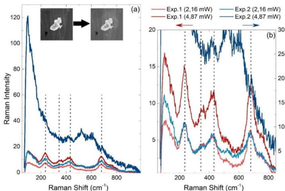
Fig.1. Changes in the Raman spectra and morphology of the particle  $\text{Li}_{3.95}\text{Mn}_{0.05}\text{Ti}_5\text{O}_{12}$  under the action of laser radiation. The time difference between the first (Exp. 1) and the second (Exp. 2) measurements was about two months. The dotted lines indicate the positions of the characteristic LTO peaks.
