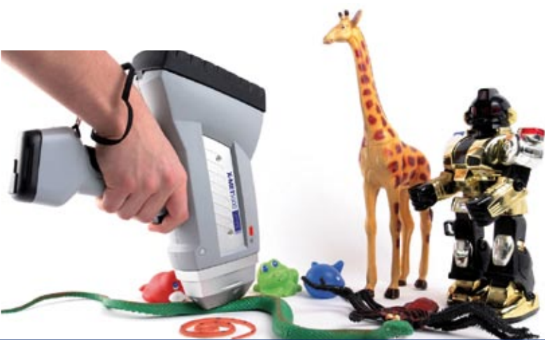
Environmental health concerns, for example, lead in toys are addressed with hand-held metal analysers
